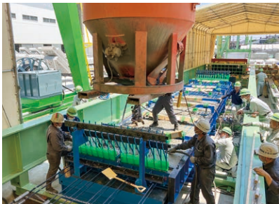
Making prototypes of prestressed concrete floor slabs
